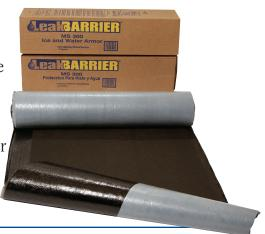
**USAGE** LeakBarrier MS300 Ice and Water Armor helps to protect a building's deck or internal structure against leaks caused by ice and water damming and wind-driven rain. It is highly effective in critical roofing areas such as valleys, ridges, coping joints, chimneys, vents, dormers, skylights and low-slope sections.
